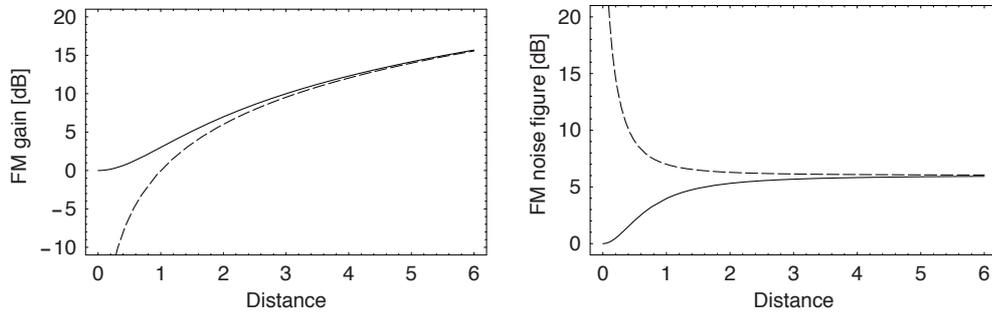
Fig. 6. Gains and noise figures of a four-mode process with quadratic gain, for cross-polarized pumps in a fiber with random birefringence ( $\epsilon = 1$ ). The solid curve represents the 1- signal, and the long-dashed curves represent the 1+, 2- and 2+ idlers. Distance is normalized to the characteristic length  $(\gamma P)^{-1}$ .
