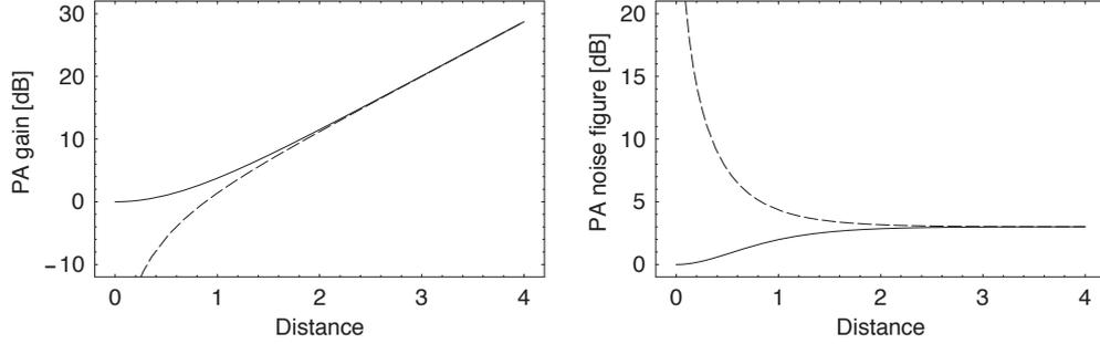
Fig. 2. Gains and noise figures of a two-mode parametric amplifier. The solid curves represent the signal, whereas the dashed curves represent the idler. Distance is normalized to the gain length  $[\gamma\epsilon(P_1 P_2)^{1/2}]^{-1}$ .
