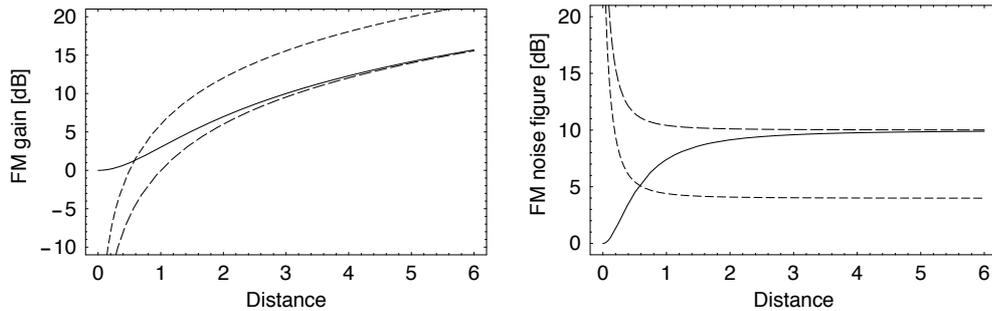
Fig. 4. Gains and noise figures of a four-mode process with quadratic gain, for co-polarized pumps ( $\varepsilon = 2$ ). The solid and long-dashed curves represent the 1- signal and 1+ idler, respectively, and the medium-dashed curves represent the 2- and 2+ idlers. Distance is normalized to the characteristic length  $(\gamma P)^{-1}$ .
