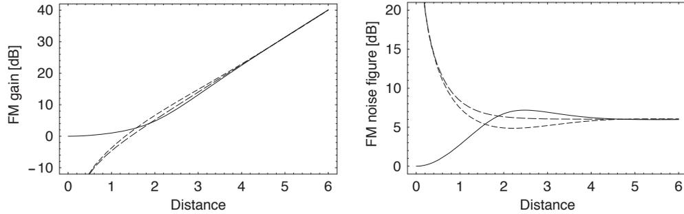
Fig. 7. Gains and noise figures of a four-mode process with exponential gain, for cross-polarized pumps in a fiber with random birefringence ( $\epsilon = 1$ ). The solid curves represent the 1- signal, the long-dashed curves represent the 1+ and 2+ idlers, and the medium-dashed curves represent the 2- idler. Distance is normalized to the gain length  $(2\gamma P)^{-1}$ .
