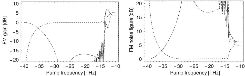
Fig. 10. Transmissions and noise figures of a four-mode process driven by cross-polarized pumps in a fiber with random birefringence ( $\epsilon = 1$ ), plotted as functions of the pump frequency  $\omega_1$ . The long-dashed curves represent the 1+ signal, and the solid, medium- and short-dashed curves represent the 1-, 2- and 2+ idlers, respectively. Frequencies are measured relative to the zero-dispersion frequency of the fiber.
