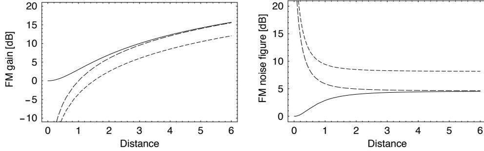
Fig. 5. Gains and noise figures of a four-mode process with quadratic gain, for cross-polarized pumps in a fiber with constant birefringence ( $\epsilon = 2/3$ ). The solid and long-dashed curves represent the 1- signal and 1+ idler, respectively, and the medium-dashed curves represent the 2- and 2+ idlers. Distance is normalized to the characteristic length  $(\gamma P)^{-1}$ .
