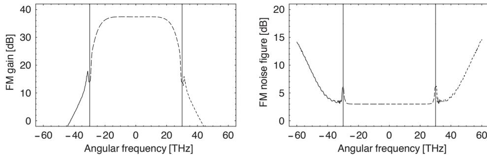
Fig. 9. Gains and noise figures of a four-mode process driven by cross-polarized pumps in a fiber with random birefringence ( $\epsilon = 1$ ). The long-dashed curves represent the 1+ signal, and the solid, medium- and short-dashed curves represent the 1-, 2- and 2+ idlers, respectively. Frequencies are measured relative to the zero-dispersion frequency of the fiber. The vertical lines denote the pump frequencies.
