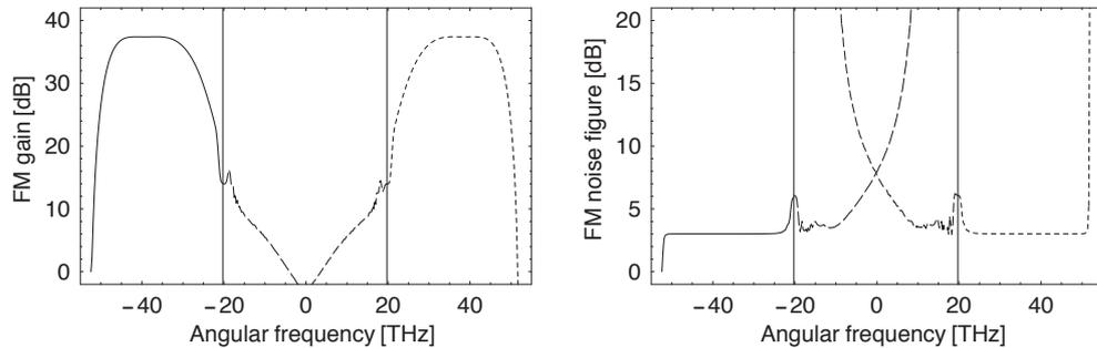
Fig. 8. Gains and noise figures of a four-mode process driven by cross-polarized pumps in a fiber with random birefringence ( $\epsilon = 1$ ). The solid curves represent the 1- signal, and the long-, medium- and short-dashed curves represent the 1+, 2- and 2+ idlers, respectively. Frequencies are measured relative to the zero-dispersion frequency of the fiber. The vertical lines denote the pump frequencies.
