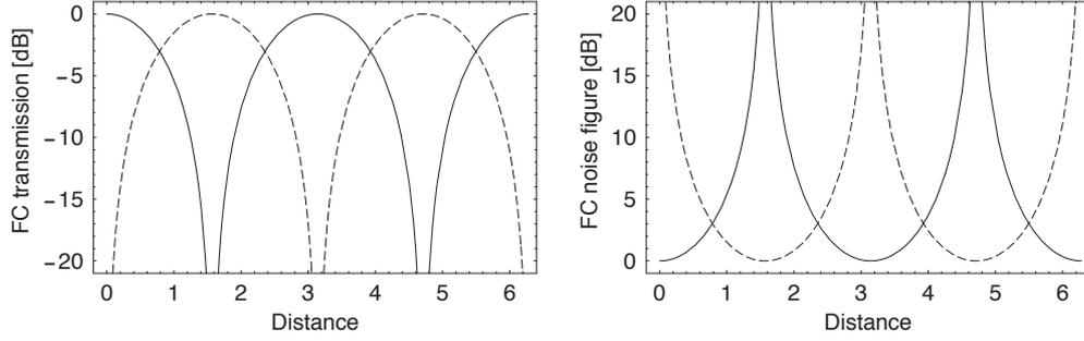
Fig. 3. Transmissions and noise figures of a two-mode frequency converter. The solid curves represent the signal, whereas the dashed curves represent the idler. Distance is normalized to the interaction length  $[\gamma\epsilon(P_1P_2)^{1/2}]^{-1}$ .
