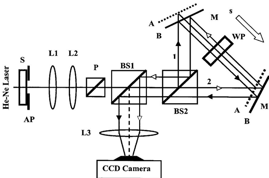
Figure 1. The surface of the source (S), primary or secondary, is imaged using three lenses onto a CCD camera. The light enters the interferometer (BS1 and BS2 are non-polarizing 50/50 beam splitters), which measures the spatial coherence function (SCF) of the transmitted light. M, mirror; P, linear polarizer; L1, L2, L3, lenses; AP, aperture; WP, wave plate set.
