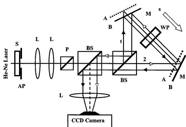
FIG. 1. Laser light passes through the scattering medium (S) whose output face is imaged using three lenses onto a charge-coupled device (CCD) camera. The output light enters the interferometer (BS = nonpolarizing 50/50 beam splitters), which measures the SCF of the transmitted light. M, mirror; P, polarizer; L, lens; AP, 1 mm aperture; WP, wave plate set.
