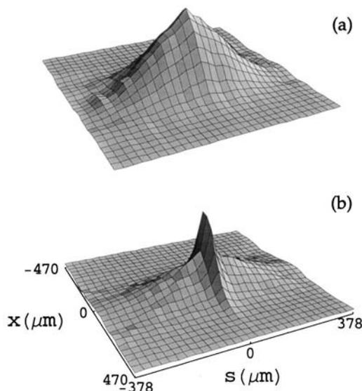
FIG. 2. Measured SCF,  $\langle \psi(x + s/2)\psi^*(x - s/2) \rangle$ , versus shear  $s$  and position  $x$ . In (a) [(b)] the volume fraction of the spheres in the medium is 0.4% (2%), corresponding to 0.27 (1.36) average scattering events.
