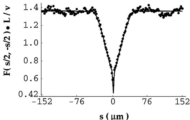
FIG. 3. Measured averaged decoherence rate times medium-transit time  $L/v$  versus separation (transverse shear)  $s$  for scatterer volume fraction 2%. Circles are measured; solid curve is theory.
