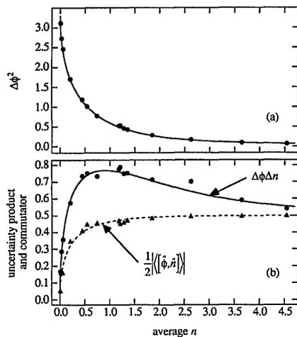
Fig. 2. (a) Variance of the phase plotted against the average number of photons in a coherent state. The points are the experimentally determined values, and the solid curve is calculated from the theory for the Pegg-Barnett phase definition. (b) Points are experimentally determined values for the uncertainty product (circles) and the commutator expectation (triangles). The curves are the theoretical values for the uncertainty product (solid curve) and the commutator expectation (dashed curve).
