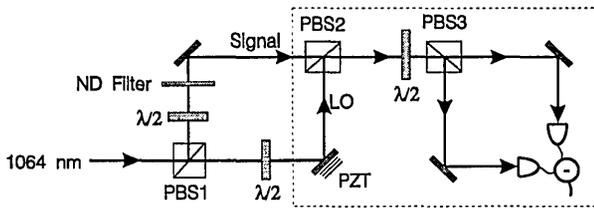
Fig. 1. Experimental apparatus. The dashed lines enclose the balanced homodyne detector.
