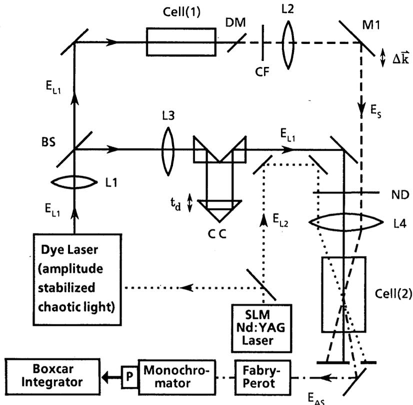
Fig. 2. Experimental setup. Stokes light generated in Raman generator Cell(1) is phase correlated to pump-laser field  $E_{L1}$ . The pump field is delayed by time  $t_d$  and combined with probe field  $E_{L2}$  in Cell(2). The anti-Stokes spectrum is measured with a Fabry-Perot interferometer and photodiode P: BS, beam splitter; DM, dichroic mirror; CF, colored-glass filter; ND, neutral-density filter; CC, corner cube; M1, mirror; L1-L4, lenses.
