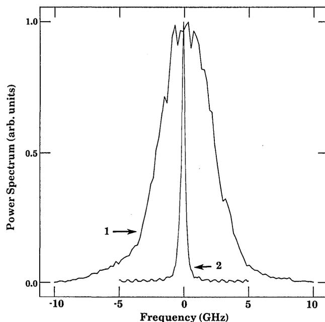
Fig. 3. Measured average power spectra of (curve 1) pump laser and (curve 2) the generated anti-Stokes field, for the case of zero Raman detuning (both cells at 48 atm). The narrow width of the anti-Stokes field illustrates the cancellation of the laser and Stokes phase fluctuations. The curves are normalized to a peak height of unity, and the horizontal scale is with respect to the center frequency of each field.
