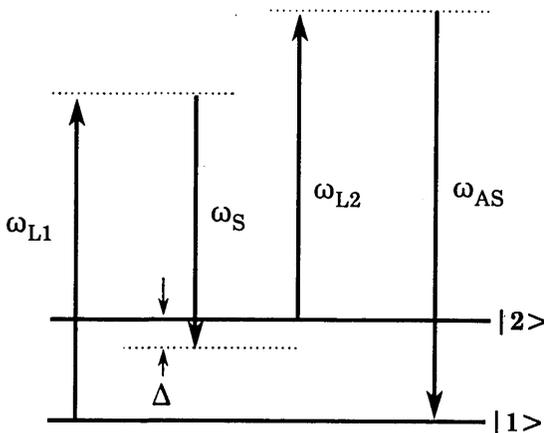
Fig. 1. Illustration of the CARS process. The frequencies (in radians per second) of pump laser  $\omega_{L1}$ , generated Stokes field  $\omega_S$ , monochromatic probe field  $\omega_{L2}$ , and anti-Stokes field  $\omega_{AS}$  satisfy  $\omega_{L1} + \omega_{L2} = \omega_S + \omega_{AS}$ . The detuning from Raman resonance is  $\Delta = \omega_{21} - \omega_{L1} + \omega_S$ , where  $\omega_{21}$  is the Raman shift of the medium.
