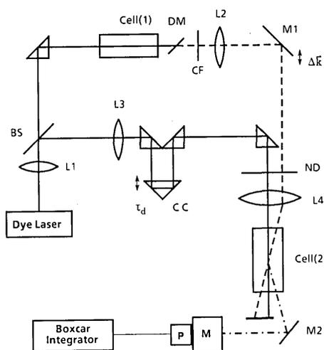
Fig. 1. Experimental setup. BS, beam splitter; DM, dichroic mirror; CF, colored-glass filter; L1-L4, lenses; ND, neutral-density filter; Cell (1), Raman generator cell; Cell (2), CARS cell; M1, M2, mirrors; M, monochromator; P, photodiode; CC, corner cube.
