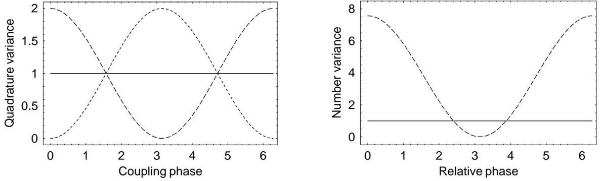
Figure 3: Signal quadrature and number variances plotted as functions of the coupling phase and relative phase, respectively. The solid lines represent phase-insensitive amplification, whereas the dashed and dotted curves represent phase-sensitive amplification. In (a) the dashed curve represents the  $x$  variance, whereas the dotted curve represents the  $y$  variance.
