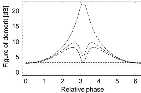
Figure 12: Figures of demerit for PC followed by FC. The solid, long-, medium- and short-dashed, and dotted curves represent  $T = 1.00, 0.75, 0.50, 0.10$  and  $0.00$ , respectively.
