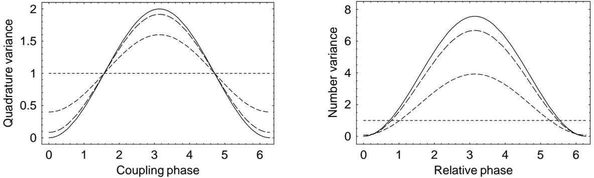
Figure 8: Signal quadrature and number variances plotted as functions of the coupling phase and relative phase, respectively. The solid, long- and short-dashed, and dotted curves represent  $T = 0.5, 0.3, 0.1$  and  $0.0$ , respectively.
