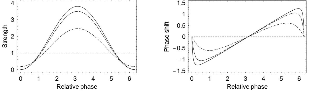
Figure 7: Signal strength and phase shift plotted as functions of the relative phase. The solid, long- and short-dashed, and dotted curves represent  $T = 0.5, 0.3, 0.1$  and  $0.0$ , respectively.
