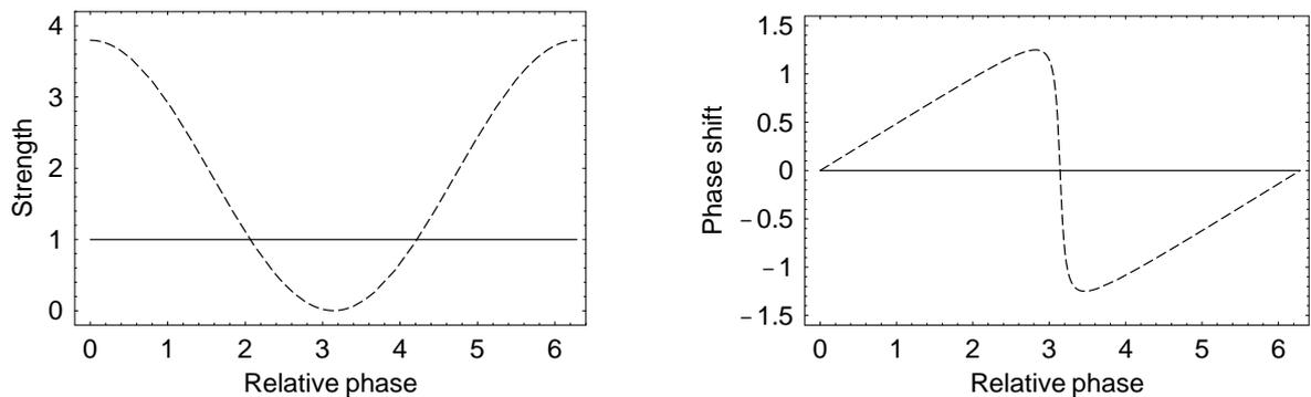
Figure 2: Signal strength and phase shift plotted as functions of the relative phase. The solid lines represent phase-insensitive amplification, whereas the dashed curves represent phase-sensitive amplification.
