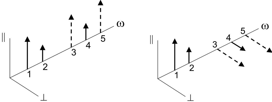
Figure 6: Polarization diagrams for cascaded scalar and vector FC and PC. During FC pump 3 is on and pump 5 is off, whereas during PC pump 3 is off and pump 5 is on.
