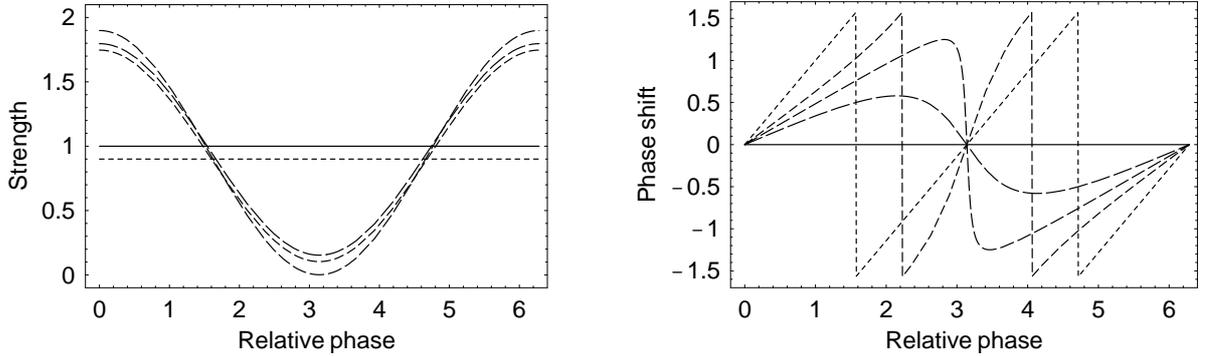
Figure 10: Signal strength and phase shift plotted as functions of the relative phase. The solid, long-, medium- and short-dashed, and dotted curves represent  $T = 1.00, 0.75, 0.50, 0.10$  and  $0.00$ , respectively.
