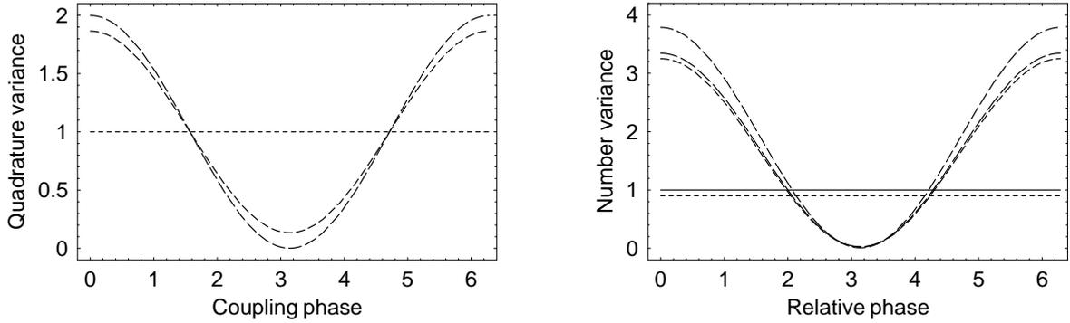
Figure 11: Signal quadrature and number variances plotted as functions of the coupling phase and relative phase, respectively. The solid, long-, medium- and short-dashed, and dotted curves represent  $T = 1.00, 0.75, 0.50, 0.10$  and  $0.00$ , respectively.
