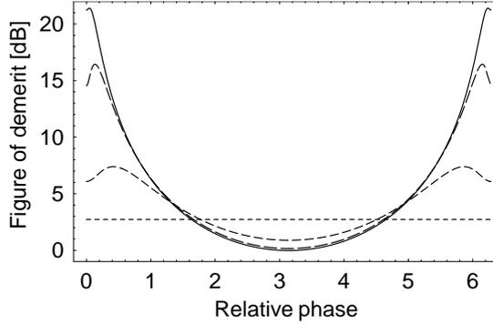
Figure 9: Figures of demerit for degenerate vector FWM. The solid, long- and short-dashed, and dotted curves represent  $T = 0.5$ ,  $0.3$ ,  $0.1$  and  $0.0$ , respectively.
