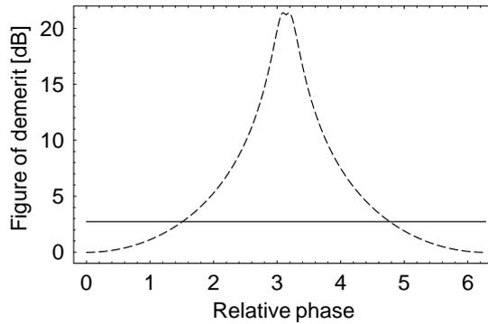
Figure 4: Figures of demerit for phase-insensitive amplification (solid line) and phase-sensitive amplification (dashed curve) plotted as functions of the relative phase.
